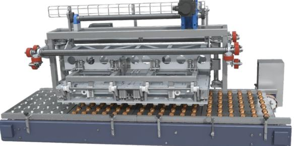
The machine is designed to remove the product from the baking sheets with its following spreading on a conveyor belt without overturning or damaging the product.
